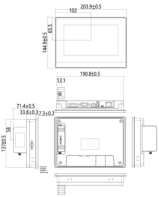
Embedded installation opening size: 192mm \* 138mm (+ 1.0 / - 0.0mm)
